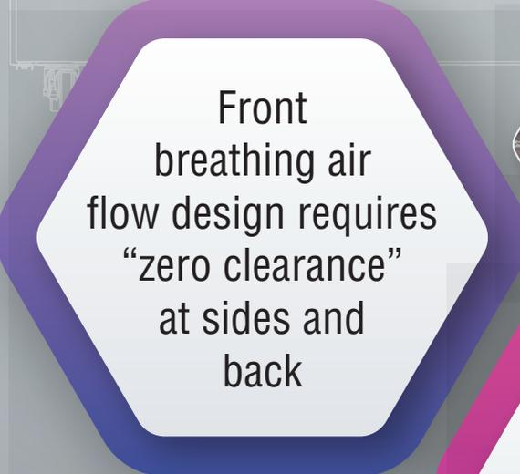
Front breathing air flow design requires “zero clearance” at sides and back
