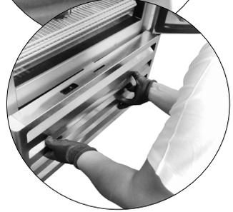
**Step 3.** Remove the two screws from the lower hinge and remove the door by pulling straight down until it is free of the upper hinge pin.
